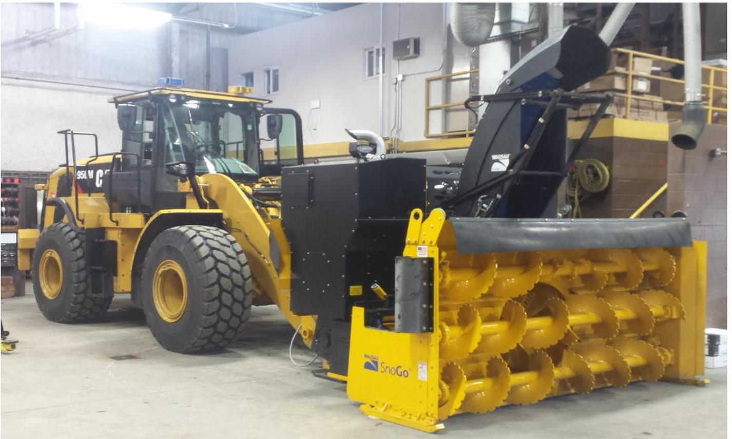
(Photo: The New Cat 950M Loader with Wausau MP 318 Snow Blower attachment at the Public Works Maintenance Facility)
