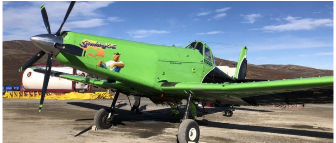
(Photo: Dromader M-18A w/ a Capacity of 12,000 lbs., 680 Gallons & Capable of 140 Knots Cruising Speed)
