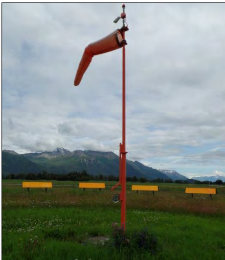
Figure 2-19. Primary Lighted Wind Cone in Segmented Circle
