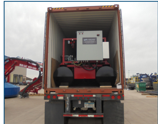
The MC-40E can be transported anywhere in the world in a 40 ft. ocean container.
