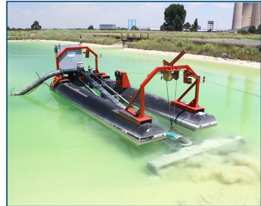
An MC-40E performs maintenance dredging on sludge lagoon.
