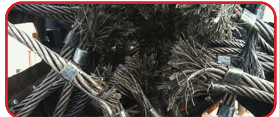
Inside of Plug Hug after 500 hydrant cleaning cycles. Notice lack of any wear on cable assemblies.
