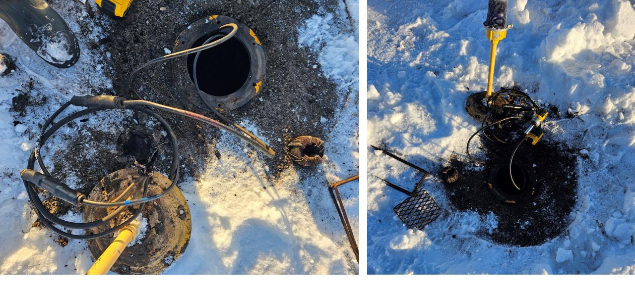
Photos of a transformer that shorted and burned underneath a taxiway edge light on the south end of the runway. It took a half day to find and bypass the burned transformer/light fixture. A contracted electrician will need to follow up and fix the discrepancy. It's likely that aging wiring and appliances contributed to the failure.
