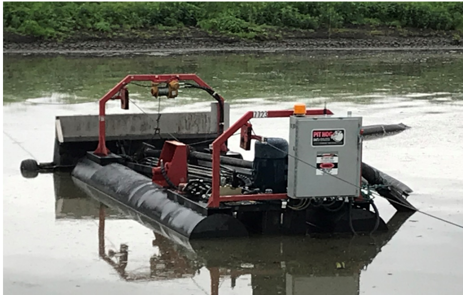
Figure 2: LWT Pit Hog RUNT Dredge
