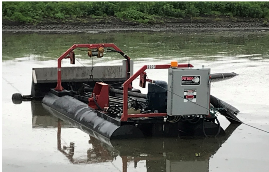
Figure 2: LWT Pit Hog RUNT Dredge
