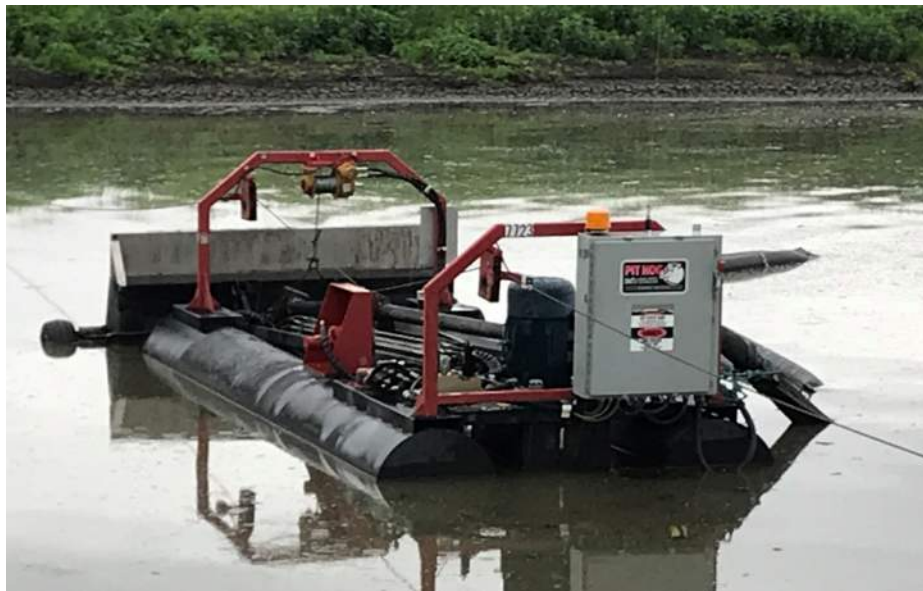
Figure 2: LWT Pit Hog RUNT Dredge
